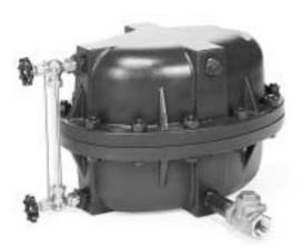
The patented Armstrong PT-104 Mini Pump Trap is the smallest non-electric solution that can move condensate or other liquids from lower to higher points and from lower to higher pressures. Condensate can be returned at temperatures well above the 210°F (99°C) limit of conventional electric centrifugal pumps without the headaches of leaking seals or cavitation problems. The PT-104 Mini Pump Trap is the small solution for a big problem.
